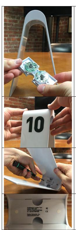
Once both circuit boards have been placed, the next step is to re-assemble the locator.
